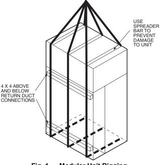
Fig. 1 — Modular Unit Rigging
